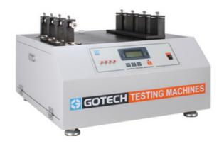
The Shoelace Abrasion Tester is designed for testing the resistance of all shoelaces to abrasion. Two shoelaces are horizontally crossed in a moveable clamp, rubbing against each other, so as to determine their abrasive resistance.
