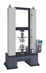
The universal tensile tester is used for performing tension, pressure or bending tests. This involves subjecting a sample to an increasing tensile load until it breaks, to determine how the material reacts to forces being applied in tension.
