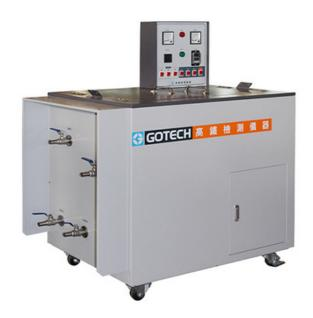
This Standard Launder Tester is used to test the washing resistance level. During the experiment, the stain specimen, the test liquid, and the steel ball are put into the test cup, washed and dried according to the specified temperature and time, and compared with the gray scale, so as to evaluate the washing resistance level of the specimen, and the washing durability test of organic solvents can also be performed.
