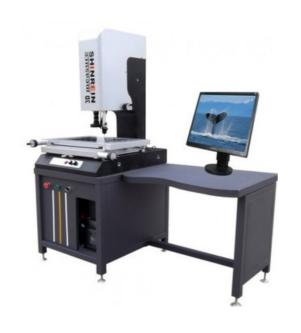
The Optical Image Measuring Instrument uses image processing technology to perform automatic measurements of products that are both fast and highly accurate. It uses highly accurate CCD cameras to enable the observation of color images, and the software associated made it possible to perform varied edge detections and to support complicated calculations.
