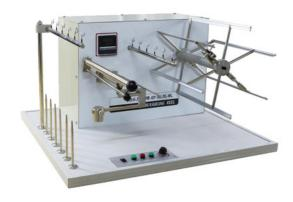
Wrap Reel, also called as Yarn Measuring Instrument, is a device for measuring yarn and making it into hanks of a standard size. The reel is of a standard size and its revolutions are counted as the yarn is wrapped around it. It is to produce skeins of yarn of a predetermined length and number of turns for count and strength testing.
