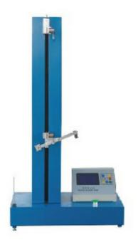
The yarn strength tester is used to measure the breaking force, elongation, and toughness properties of the yarn.
