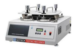
Martindale Abrasion Tester is used for testing of textile products according to Martindale's standard system and tests the abrasion resistance of the fabric through the test. Abrasion resistance refers to the resistance of a fabric to other materials in the process of repeated friction.
