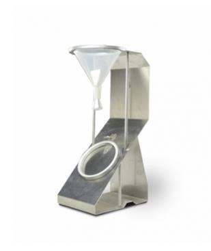
The Spray Rating Tester is for evaluating the ability of waterproof fabrics to repel water using a "shower test". The test does not measure the penetration of water through fabric, instead it determines the resistance of any fabric, which may or may not have been given a water-resistant or water-repellent finish, to surface wetting by water.
